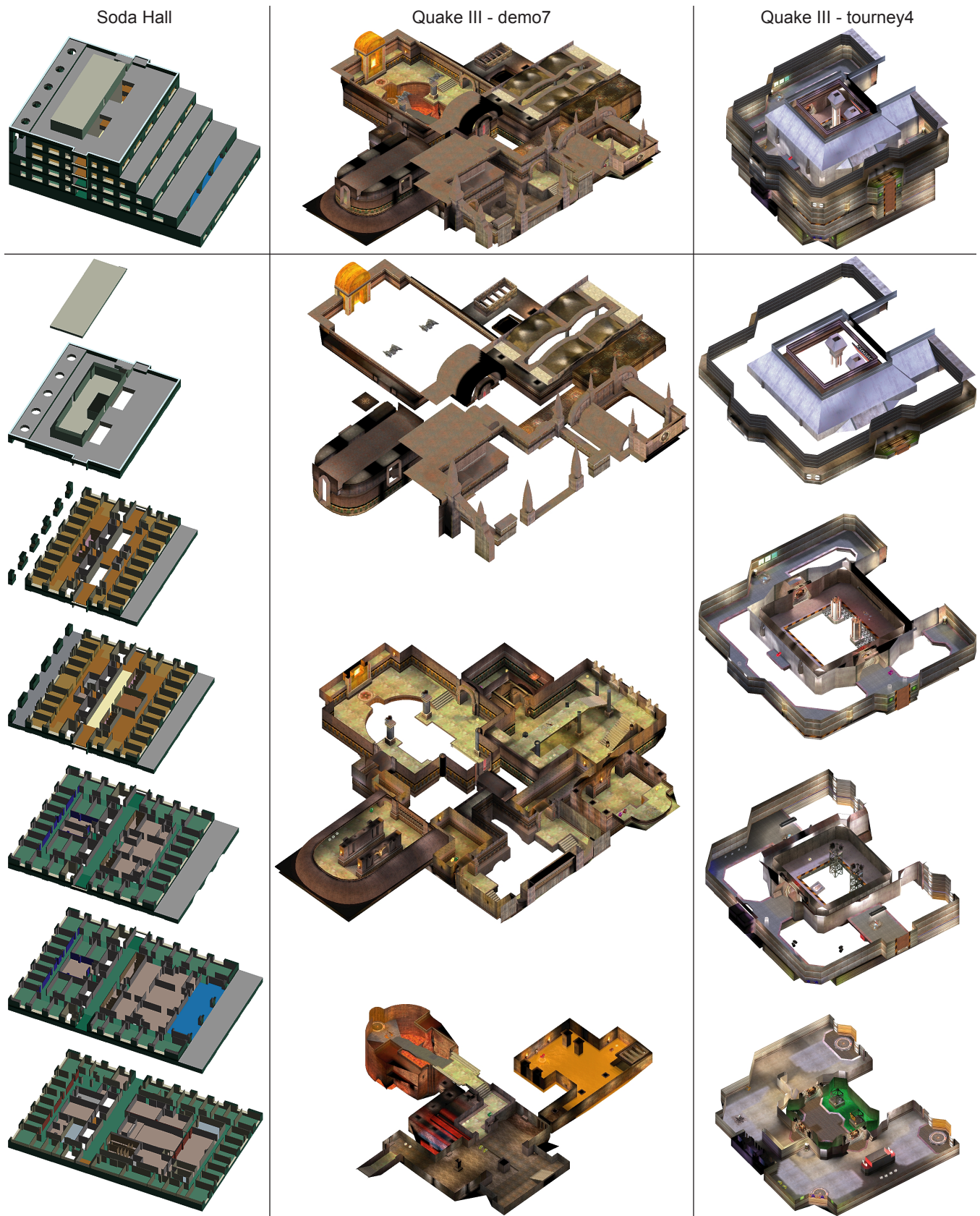
Figure 4: Exploded views generated by our system. Each column shows the environment from an external axonometric viewpoint, first unexploded and then exploded. We non-invasively modified an ArcBall viewer to generate the Soda Hall example and we modified Quake III to generate the demo7 and tourney4 examples. While the unexploded view shows external structure, the exploded view simultaneously reveals both internal and external structure.
