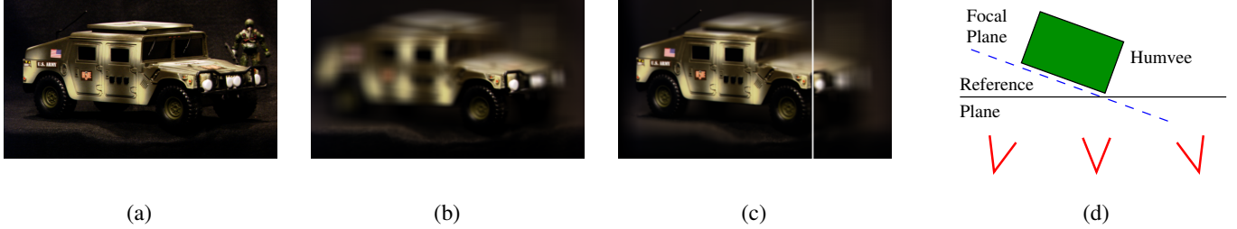
Figure 3: User-driven change of focus. (a) An image from a light field showing a toy humvee at an angle to the plane of cameras. (b) Synthetically focused image on reference plane. Note that the left side of the humvee is out of focus, since it is not on the reference plane. (c) If we rotate the focal plane about the line indicated, we can get the full side of the humvee in focus with a tilted focal plane. (d) Plan view of our setup.
