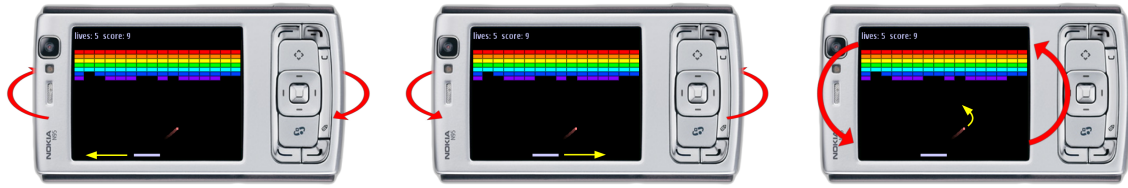
Figure 7: Viewfinder alignment acts as a continuous input on devices which otherwise lack them. This figure illustrates how horizontal translation and camera rotation are used to control a game of Breakout. Horizontal translation moves the paddle left and right, while rotation steers the ball.
