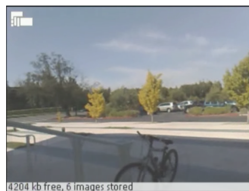
Figure 8: A screenshot from the panorama capture program. The top left shows a map of the relative locations of the 6 frames captured so far.
