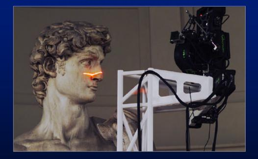
height of gantry: weight of gantry: 7.5 meters800 kilograms
