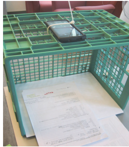
Fig. 4. Setup that was used to set up the camera station, consisting of a camera-enabled mobile phone zip-tied to a milk crate.
